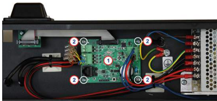
Fig. 8 Replacing a FC HUB board.
